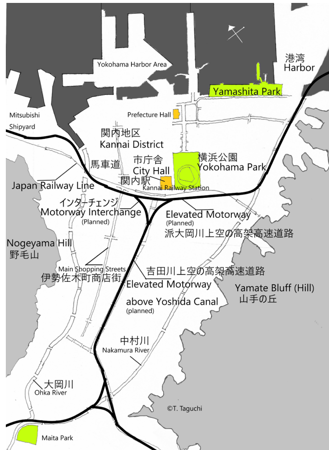
Fig.9 The initially decided plan of elevated motorway routes by MoC in 1968. Source: own elaboration.
