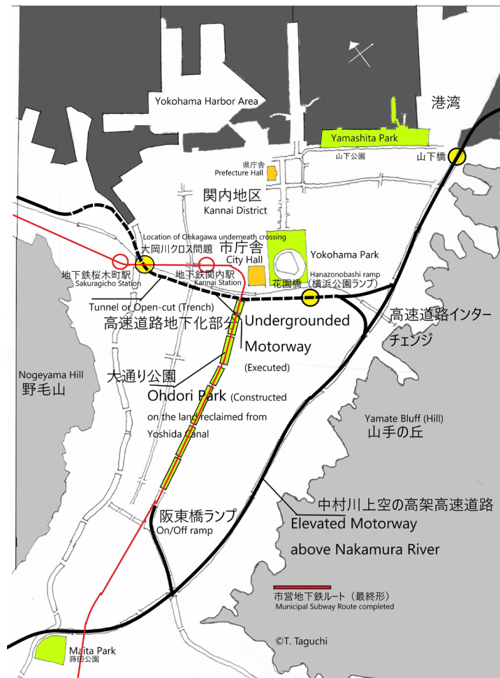
Fig.10 The finally agreed part of underground motorway (dotted line) and its connecting elevated motorways above Nakamura river. Source: own elaboration.
